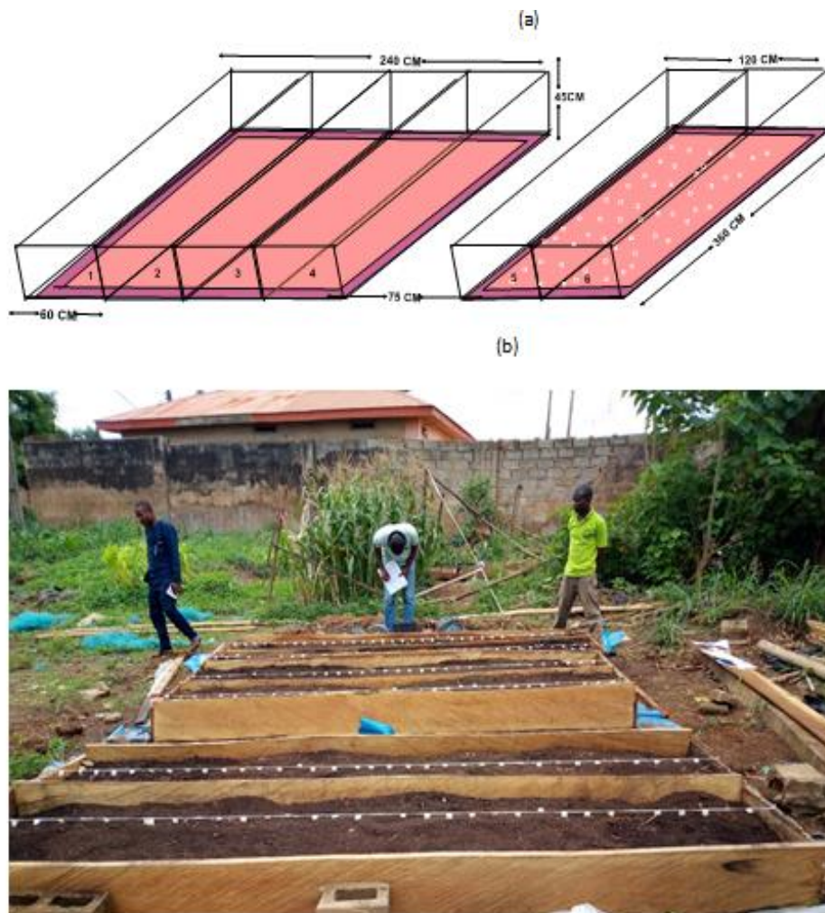
Figure 2: The design of the (a) experimental Soil Profile Box (b) constructed randomized Experimental Blocks
